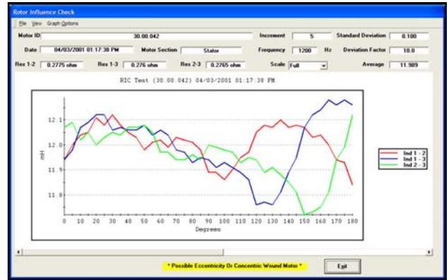
Fig. 9. Inductance test of a rotor in which the residual flux had been distorted by external influences.
