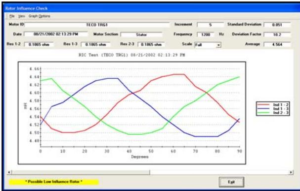
Fig. 2. Inductance test of a rotor “with Influence.”
